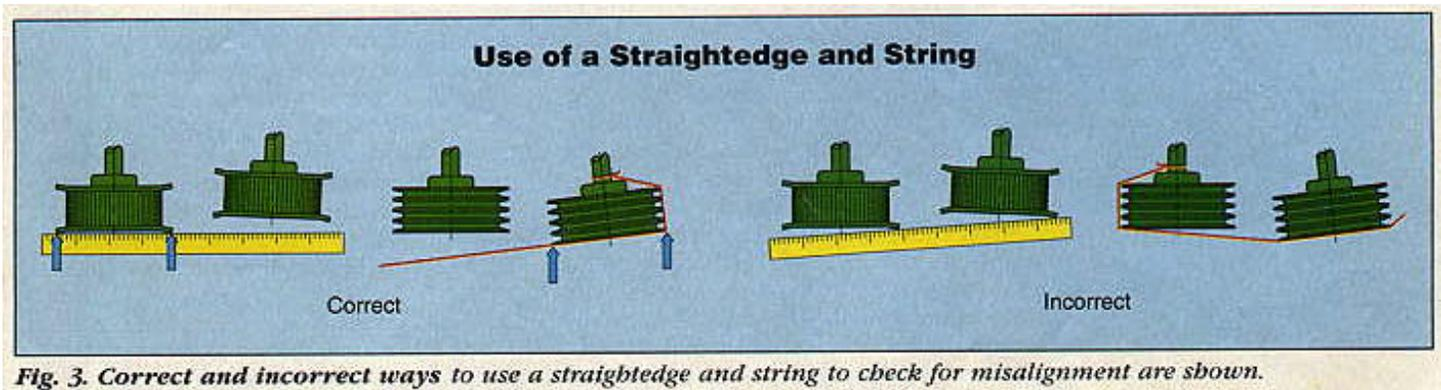
*Fig. 3. Correct and incorrect ways to use a straightedge and string to check for misalignment are shown.*
